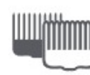
Comb Setting A : 1 to 10 mm B : 11 to 20 mm
